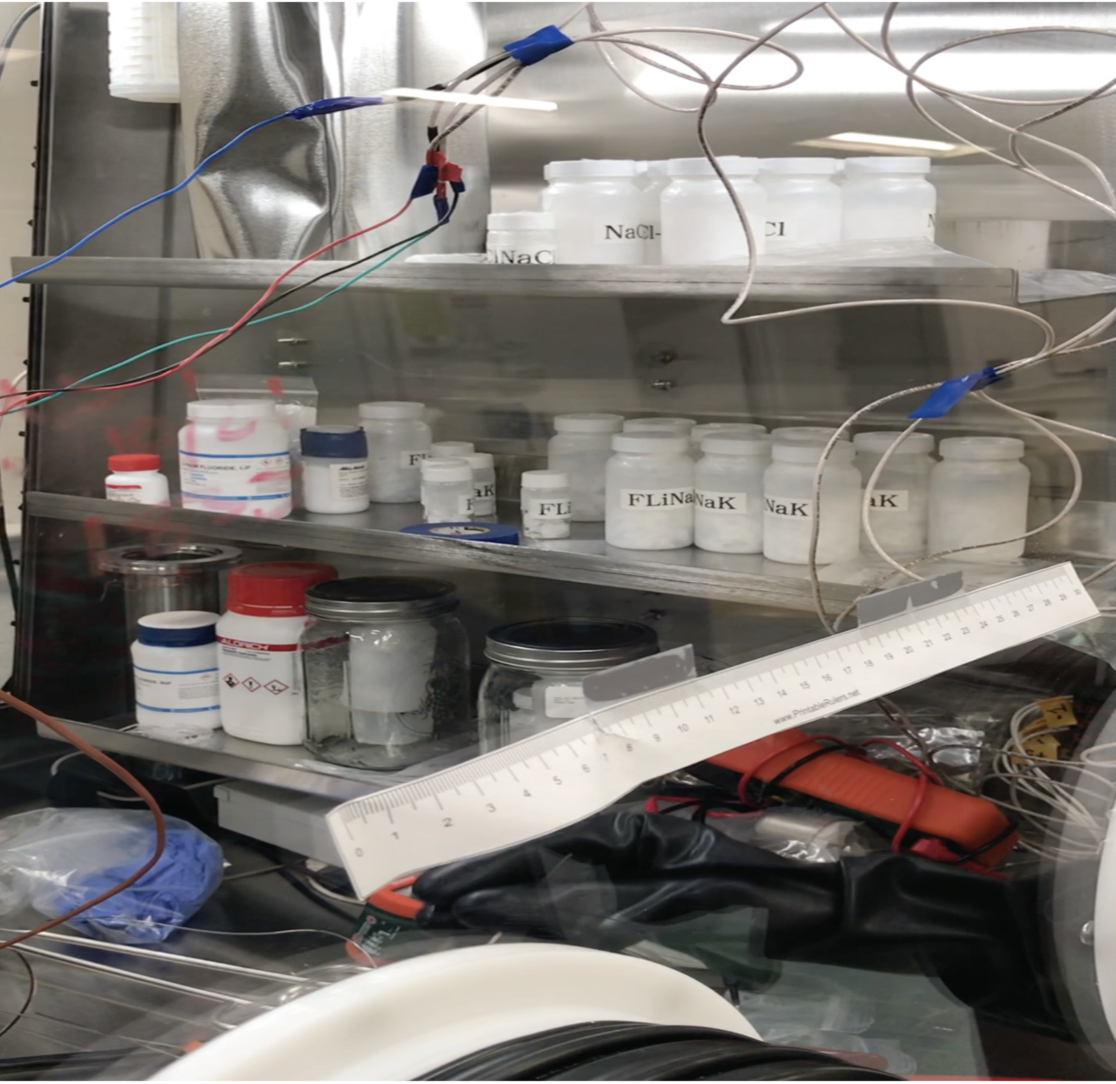
Figure 2. Salt Samples stored under inert gas within a glovebox at UC Berkeley. It is important to store the samples in an inert environment to maintain their original, as shipped from ORNL, purity.
